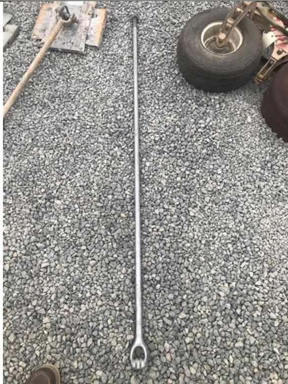
10' x 1" rod that has been cut to 79" and re-threaded
