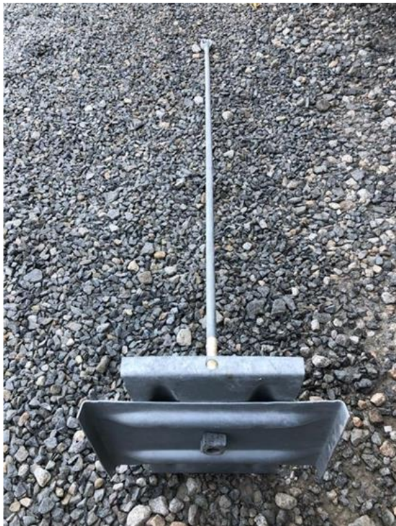
PISA with helix removed and partially threaded directly into plate anchor
