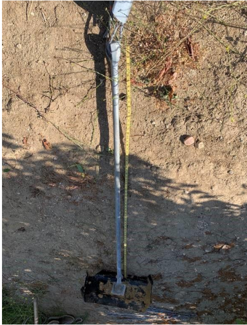
A 6' extension rod connected to plate anchor
