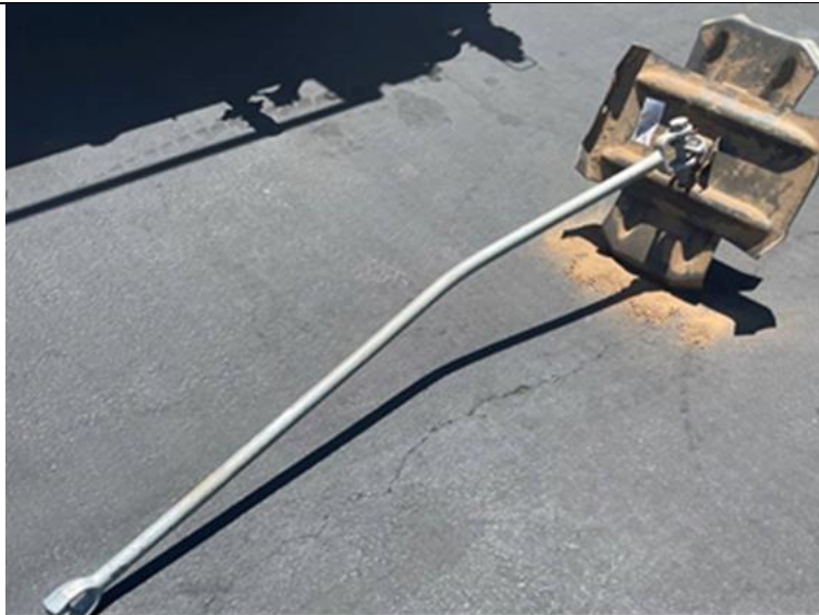
3' extension rod connected directly to a plate anchor utilizing an I-bolt
