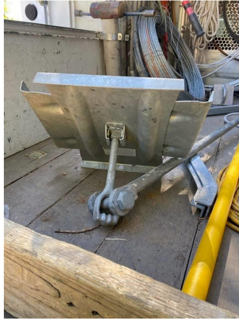
6' extension attached to modified rock anchor
