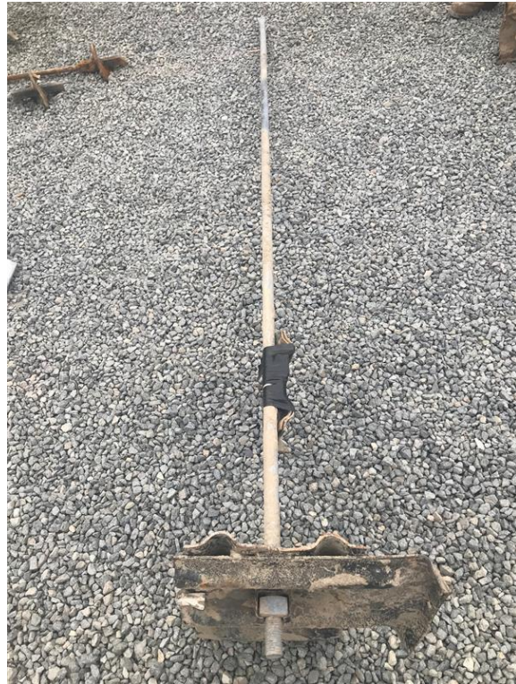
10' rod with modified plate anchor (fins cut to fit in the hole)
