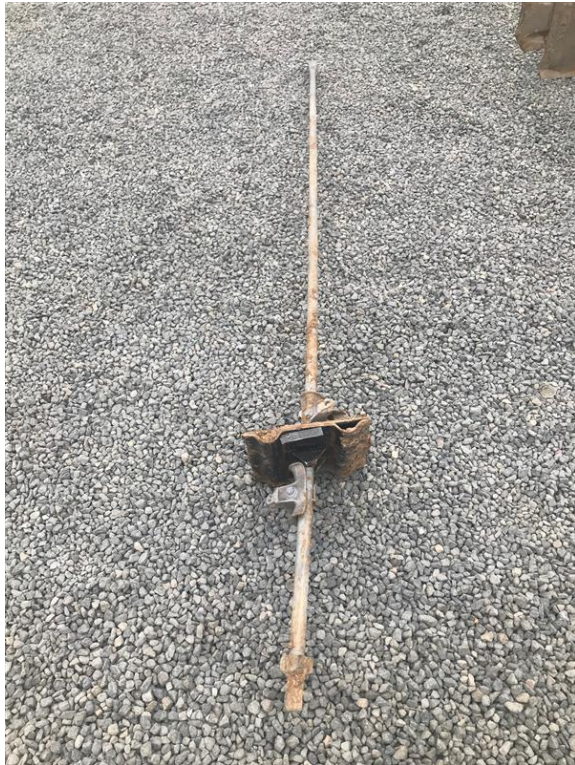
10' x 1 1/4" rod utilizing insulator clamp tops to secure plate anchor in place
