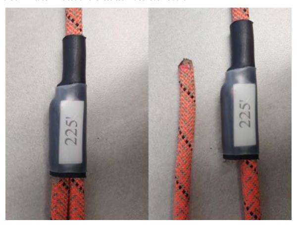
This type of rope comes from the manufacturer with a factory termination as shown in the picture below. The factory termination will always come with a clear shrink tube to allow for inspection of the termination stitching. In addition, the tag placed under the shrink tube contains the manufacture date, size, length, strength, and lot number.
